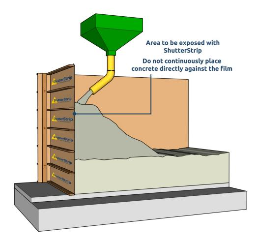
2) Do not continuously pump/place concrete directly against the area of the formwork shutter that the retarder film has been applied to. If there is no other option to this, place a strong plastic sheet over the retarder film and when the shutter is being loaded, pull the plastic sheet up accordingly, allowing the concrete to come into contact with the film. If these procedures are not followed, this could result in the film being rubbed away, leaving areas of unexposed aggregates.
